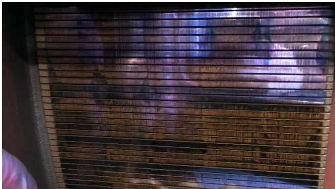
Figure 7: Contamination, vibration, and copper drag
