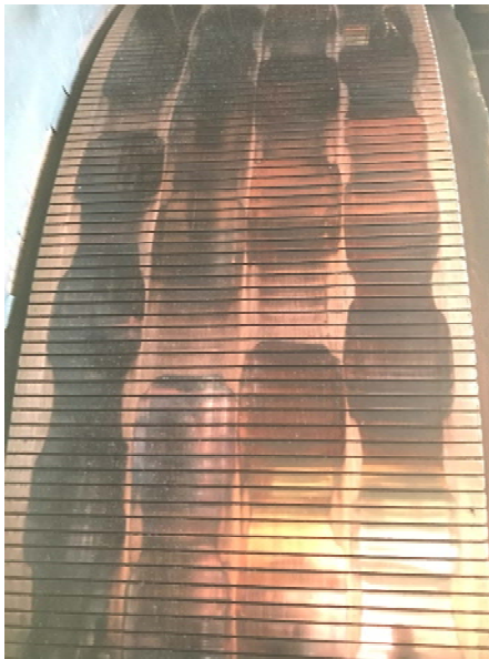
Figure 1: Regular shock loading from heavies or unprocessed bales or logs
