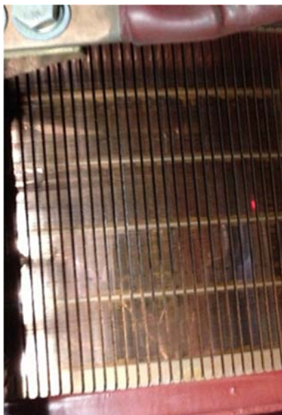
Figure 9: Acceptable condition, light film
