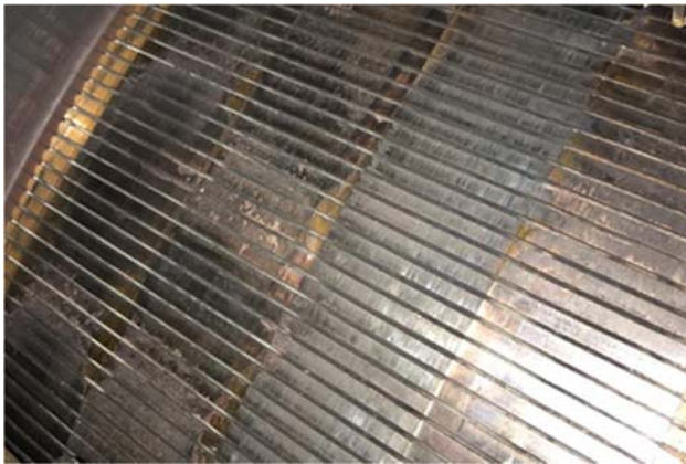
Figure 4: Long periods of high current low RPM operation in addition to photographing
